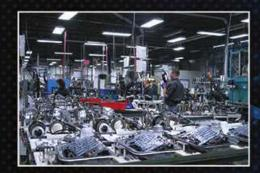
JASPER Transmissions are remanufactured in cellular environments, known as PODs, by teams specializing in a specific transmission or a family of transmissions. This approach allows for cross training and has improved the quality and efficiency of our operations to hold the line on costs and increase the availability of our transmissions for you and your customers.
