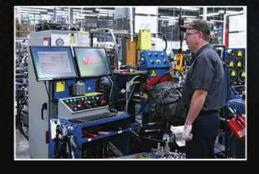
Torque Converters are dynamically balanced to eliminate vibration which can ultimately lead to transmission damage. Finally, every remanufactured JASPER automatic transmission is 100% dynamometer tested under load to ensure proper gear ratios, line pressure, cooler pressure and flow.
